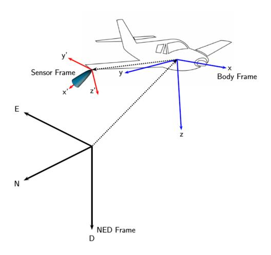
Additional coordinate frames can be required. For example, often tracks are not maintained in NED (or ENU) coordinates, as this coordinate frame changes based on the latitude and longitude where it is defined. For scenarios that cover large areas (over 100 kilometers in each dimension), earth-centered earth-fixed (ECEF) can be a more appropriate global frame to use.
